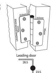
Leading door edge **Right Side** opening **Remove & invert** hinge pin
