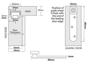
Routing of the guide wheel is **80mm** length, **16mm** width, **6mm** depth. On **34mm** & **40mm** door thickness's, centre for the guide wheel is **17mm** from the leading door face edge.
